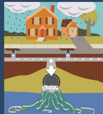
Lawn fertilizers (and other pollutants such as pesticides, oil, gasoline, antifreeze and dog waste) mix with rain and irrigation runoff, wash into storm drains on the street, and empty into local waterways, with no filtration or treatment.
