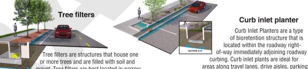
gravel. Tree filters are best located in narrow right-of-way areas where space is limited. Typical locations include medians, streetscapes, shoulders, and along shared paths.
